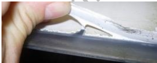
Figure 33 Examples of sealant failure.
