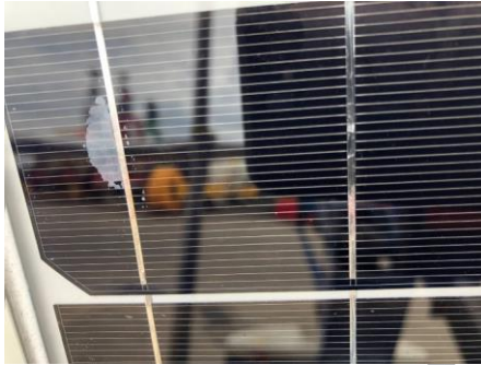
Figure 39 Delamination on a new solar module
