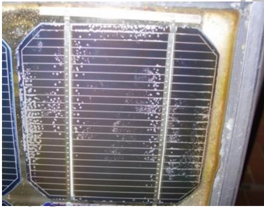
Figure 31 Cell corrosion.
