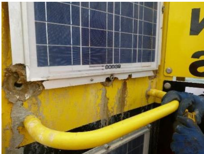
Figure 36 Impact of leakage current
