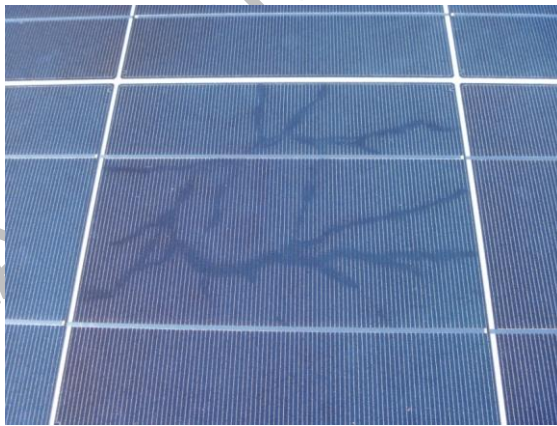
Figure 28 An example of Snails trails on a solar module (from the internet).
