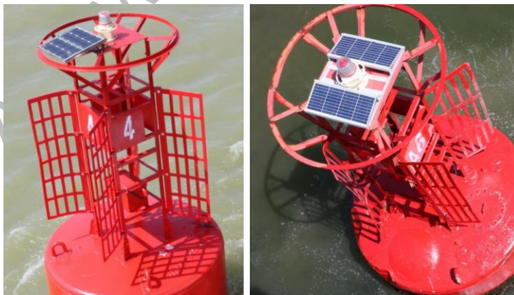
Figure 24 Wind impact to solar modules on buoys
