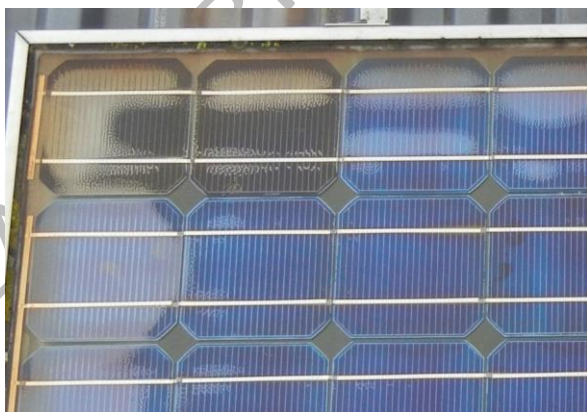
Figure 35 Encapsulant discolouration
